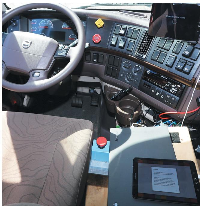
*In the cab of a truck equipped with Cooperative Adaptive Cruise Control technology, drivers monitor an interface tablet screen at left. A shut-off device, with red button, is positioned at center.*
